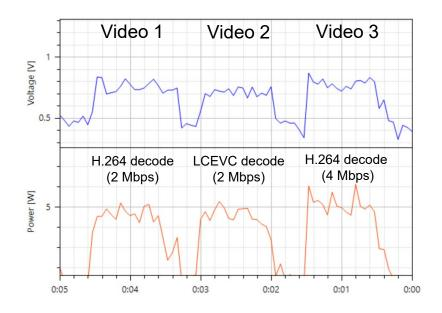
As you can see, compared to the 2 Mbps H.264 file, **LCEVC** decode consumes lower voltage and about the same power, so overall, LCEVC decode consumes less battery power. Compared to the 4 Mbps H.264 file, which is the same approximate quality as the LCEVC file, **LCEVC** playback is more efficient in both power and voltage.
